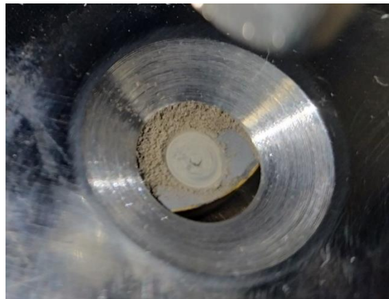
Figure 12. The worn area of the specimen with the massive wear debris at the end of the Trial_6 test. The debris partially drifted out of the worn area, then fell into the container below the specimen due to the high rotational speed.
