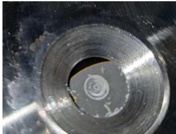
Figure 16. The worn area of the specimen with the residue of wear debris distributed along the circumference of the clamping ring during the Trial_8 test.
