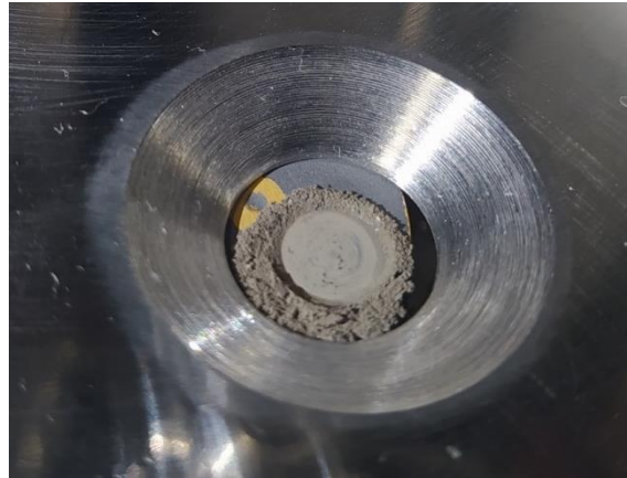
Figure 8. The worn area on the specimen for the Trial_4 with the wear debris; (note the amount of wear debris after 60 m of sliding distance).
